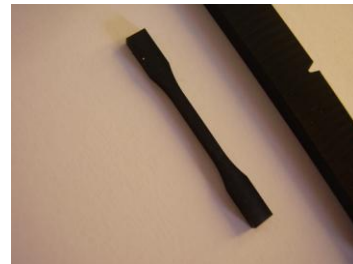
Typical tensile and IZOD impact test samples.
